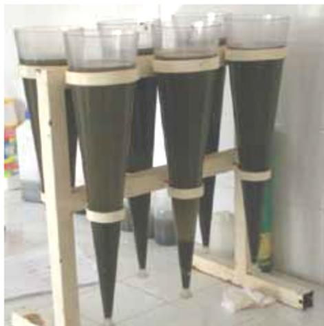
*Figure 49: Imhoff Cones To Be Used for Determination of Sludge Volume Index*
