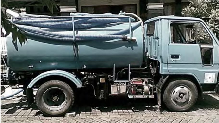
Figure 39: Vacuum Truck with Complete Equipment<sup>41</sup>
