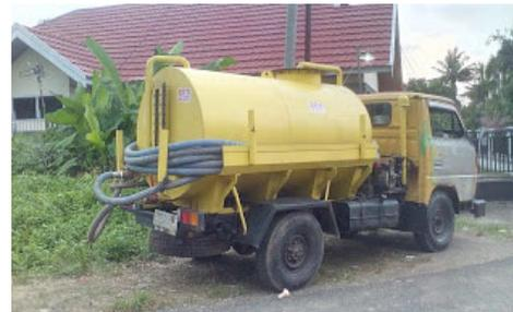
Figure 62: Desludging Equipment Operated by the Jambi Waste Hauler Companies
