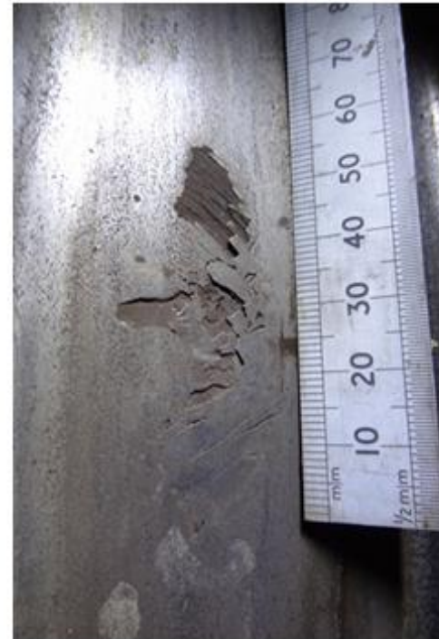
Wheel Flat / Spall
