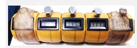
The MMDA TEC has limited capabilities in using video data to count different types of traffic moving through an intersection, so the team does this manually using field counters.
