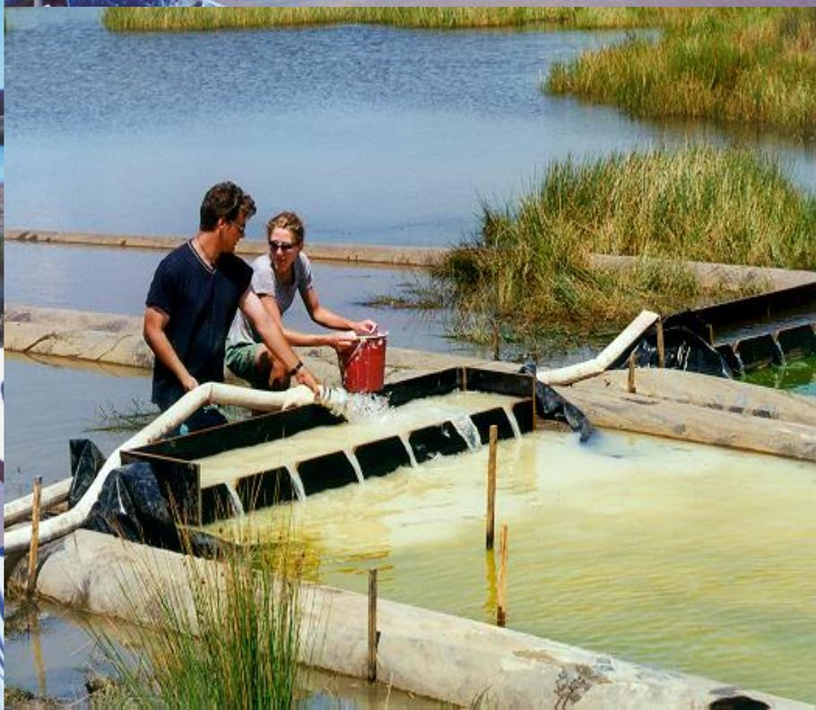
2.25 hectare Catchment Area. Rainfall runoff collected from roads and roofs to be purified before release into waterways and infiltration into watertable.
