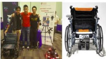
A self-guided motorized wheelchair, powered by Intel NUC, empowering elderly users to navigate autonomously, ability to detect and avoid obstacles to ensure user's safety and trigger alerts to caregiver to provide additional assistance.
