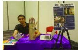
A prosthetic hand prototype with motion sensing by a glove . Users will wear a glove and moving fingers will move the servos to act like muscles using flex systems. Future plans to explore using EMG Sensing.
