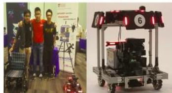
A fully autonomous base Robot with path planning, vision detection capabilities using Intel NUC.
