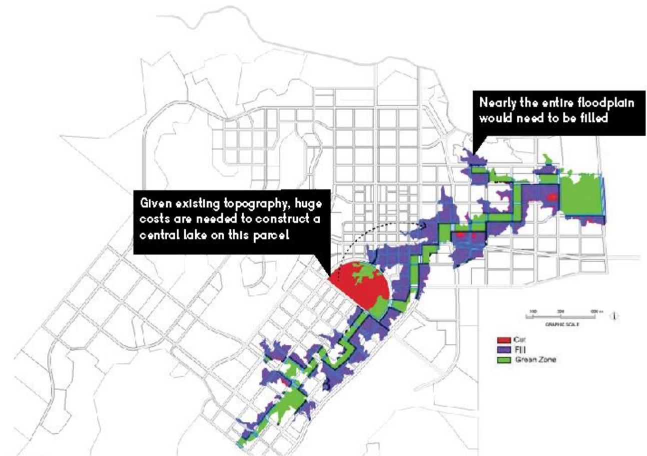
Figure 7. Master plan grading implications.
