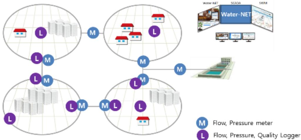
Establishing **DMA** and building a **water network model** and **D/B** by digitalizing data
