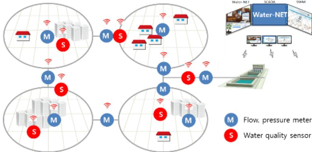
Upgrade water network with **wireless sensors and meters**
