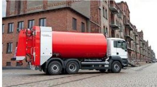
concrete agitator truck. Therefore the only moving parts are the roller bearings and one motor to drive the cylinder. When the waste has to be emptied from the cylinder, the motor is merely reversed and this spiral plate forces the waste from the vehicle. Such systems are becoming more popular throughout Europe and require far less maintenance than a typical waste compactor vehicles using the traditional ram system.
