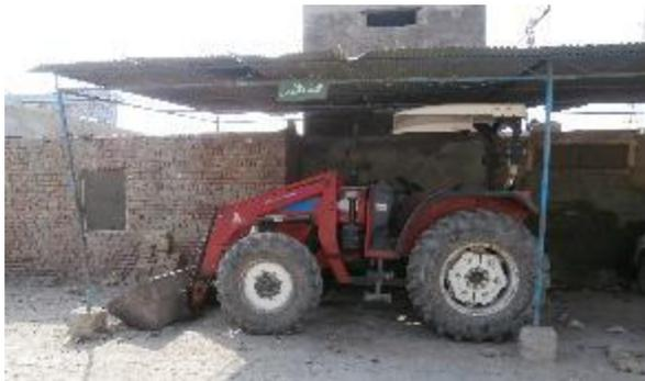
Some tractors are equipped with a front bucket that can lift the waste from the primary dumping locations into the trailer which is a significant labour saving benefit. Adding the loader element to the tractor adds more hydraulics and is now comparable to a skip bin truck excluding the body compaction elements.
