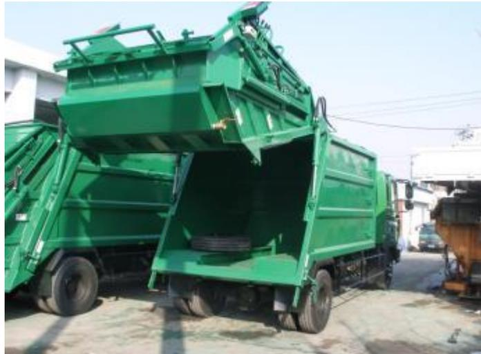
The compactors can also be fitted with arms to lift pushcarts or small skip bins into the rear trough, if those systems are proposed for primary dumping locations in some areas of the municipality rather than door to door collection.
