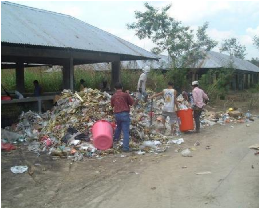
Waste piles from the loads being mixed together. Plastic buckets filled waste from one pile are mixed with the waste in other piles. Waste from the edges of various piles are collected and dumped onto the top of the pile. Aim is to make the overall waste pile one homogenous mixture of waste from the separate truck loads. (An excavator or end loader can be used instead if available of course)
