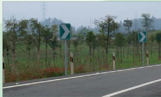
The new design includes updated safety barriers, realignments, paved shoulders, improved delineation and curve markers, enhanced skid resistance and traffic calming
