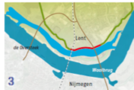
An ancillary channel is to be dug in order to give the river more room. This will create an
