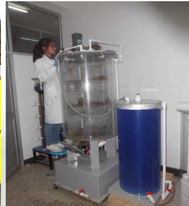
Anaerobic fermentation facilities for biomethane production (200 L)
