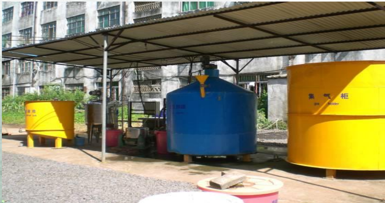
Pilot plant for biomethane production from banana stalks.
