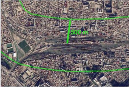
500 m buffer left/right of the railway alignment
