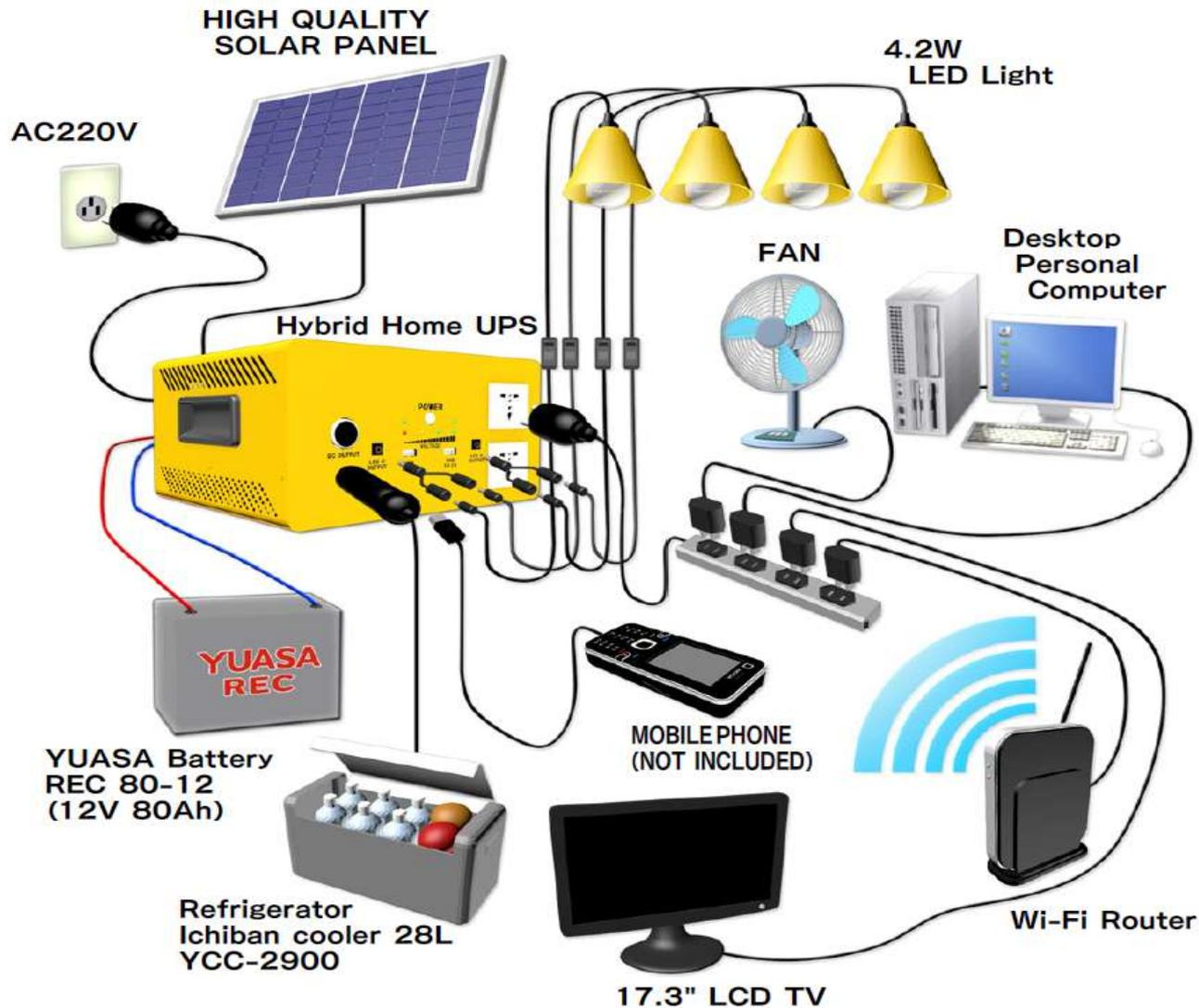
*Solar "UPS" System for small office with AVR (Automatic Volt Regulator)*
