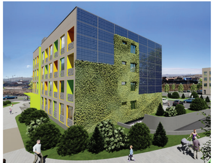
Building B – Vertical PV solar panel mixed with vertical Green wall
