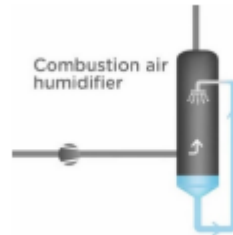
Figure 12: Combustion air humidifier, where water heated by a low-temperature source is evaporated into the combustion air flow
