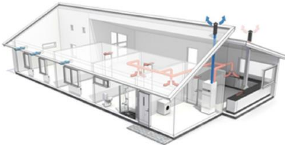
Figure 51: Ventilation air heat pump
