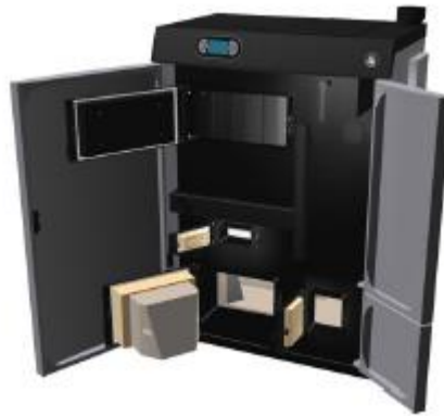
Figure 45: Double duty wood log boiler (manual stoking) prepared for mounting of pellet burner (automatic stoking)
