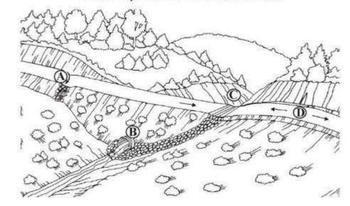
(A) Roadway Cross Drain (Dip) (B) Culvert (C) Overflow Protection Dip(D) High point in the road profile
