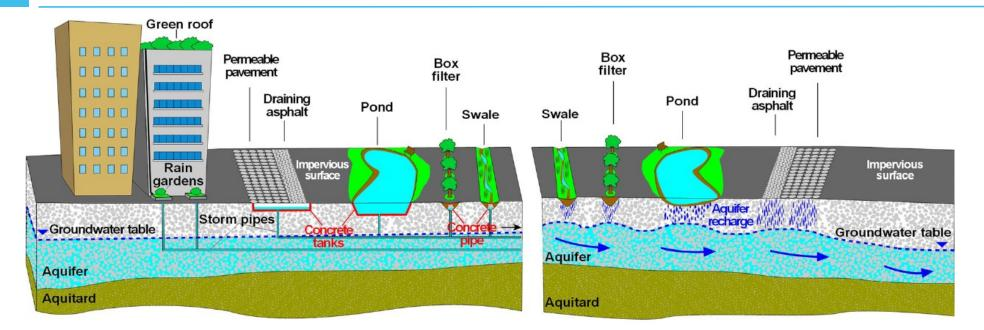
(Left) Separated drainage system for storm water collection from sewerage system for wastewater collection. (Right) Aquifer recharge management. Both techniques will absorb urban runoff and enable urban areas to adapt to climate change.
