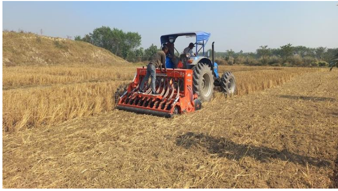
Super Seeder / Minimum-Seed Drill Can incorporate paddy straw & stubble into soil and simultaneously sow seeds
