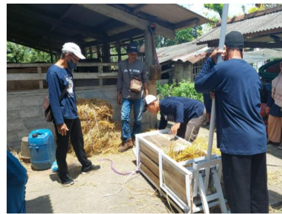
Customized Straw Pressing Machine for compact storage
