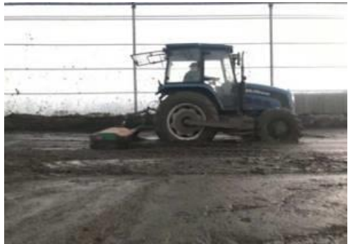
b) Cow manure composting in fertilizer processing factory (using cow manure rotator)
